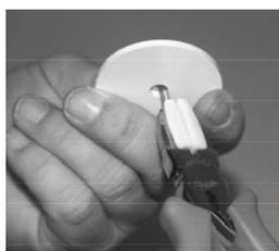
5. Pull the bit out of the chuck
