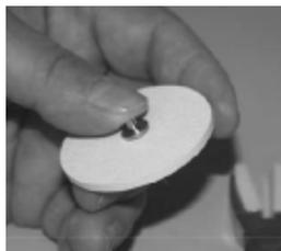
4. From the other side of the washer, grip the bit (only) by the shaft with the Nylon tipped pliers. Do not grab by the tip, use the shaft.
